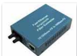
F06-FX-ST-SMXX ST 10/100M Media Converter, Single-Mode
