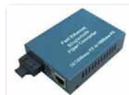
F06-FX-SC-SMXX SC 10/100M Media Converter, Single-Mode
